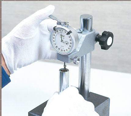
This photo shows measuring dimension of work piece by mounting dial indicator to the granite base stand.
