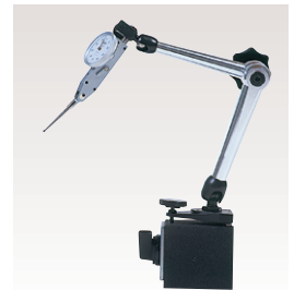
Example Magnetic Base with Test Indicator. Dial indicator is also applied.
