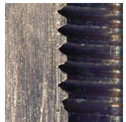
M3 Spiral Fluted Tap, ADC work, 56m/min.
