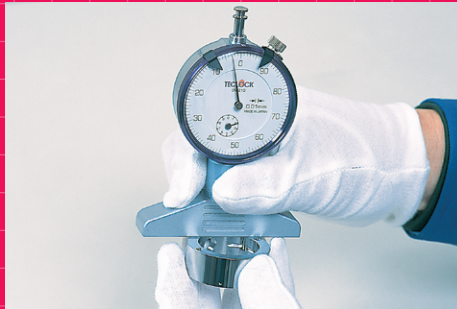
Measuring depth of concavity of work of which center is bored. The photo shows 2.03mm.
