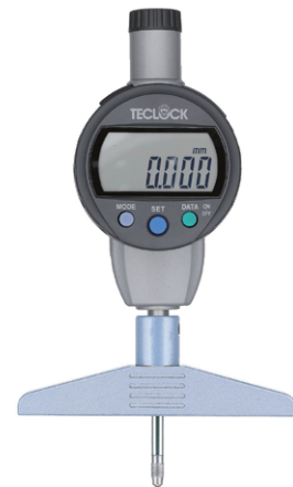
DMD-2410J φ3.2Steel Ball Contact Point Resolution 0.001mm Measuring Range 25.4mm
