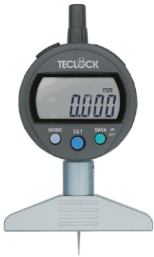
DMD-2100J Needle contact points Resolution 0.001mm Measuring Range 12mm
