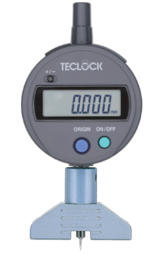
DMD-2520S2 φ3.2Steel Ball Contact Point Resolution 0.001mm Measuring Range Concave 5mm Convex4mm
