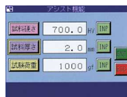
Assist function : This mode can identify the testing condition which is optimum is carried. The testing condition which is optimum can be confirmed by satisfying 2 from 3 condition of thickness, hardness, test load.
