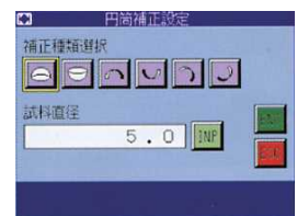
Cylindrical correction mode : This mode can set spherical surface and cylindrical correction.
