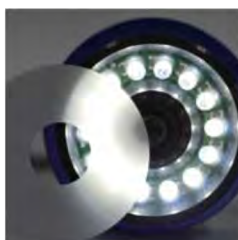
Built-in lighting (White LED) A diffusion filter is attached
