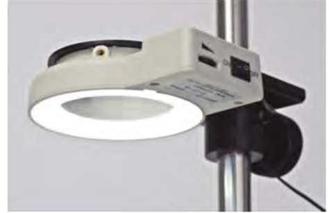
LED Ringlight with stay (A diffusion filter is attached)
